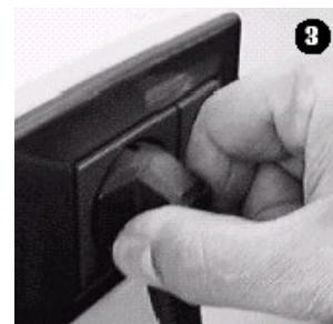
During maintenance and cleaning, or in case of bad functioning, disconnect the machine from the power plug (by pulling the plug and not the cable) (pic.2 and 3).
